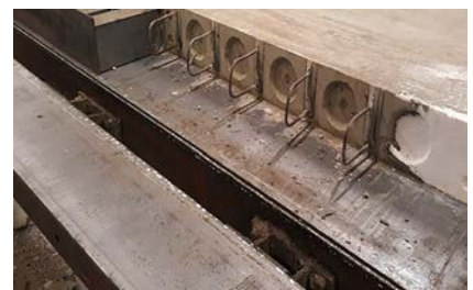
Shuttering with shear key and reinforcement penetration and finished element
